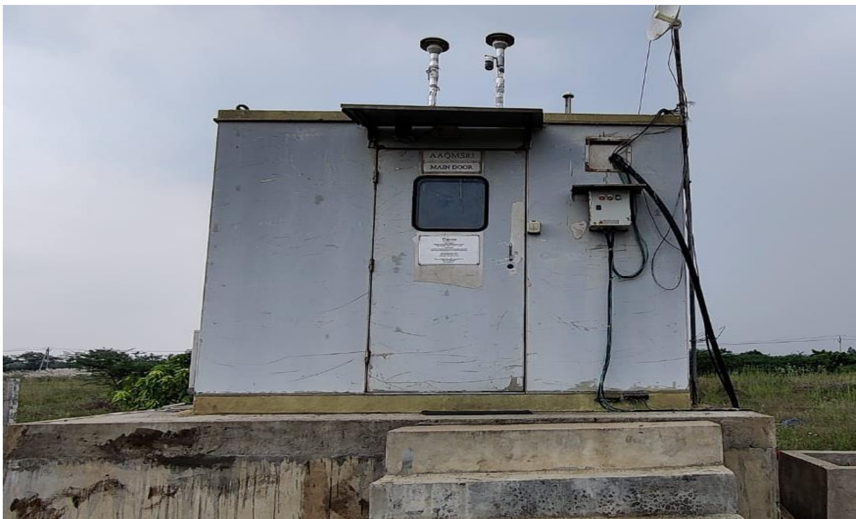
CONTINUOUS AMBIENT AIR QUALITY MONITORING STATION INSIDE THE PLANT
